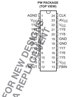
The CDC2510A is a high-performance, low-skew, low-jitter, phase-lock loop (PLL) clock driver. It uses a PLL to precisely align, in both frequency and phase, the feedback (FBOUT) output to the clock (CLK) input signal. It is specifically designed for use with synchronous DRAMs. The CDC2510A operates at 3.3-V V<sub>CC</sub> and provides integrated series-damping resistors that make it ideal for driving point-to-point loads.
